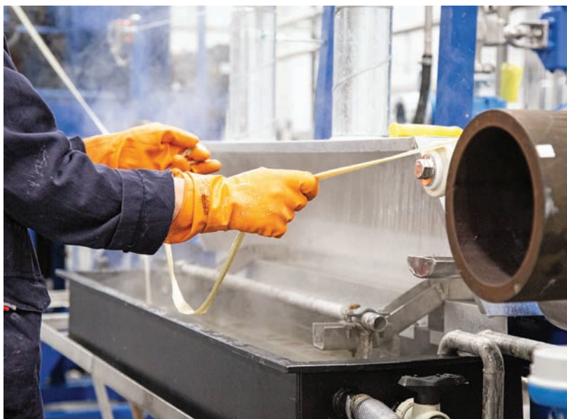
Wet spinning at one of Infinited Fiber's pilot plants.
