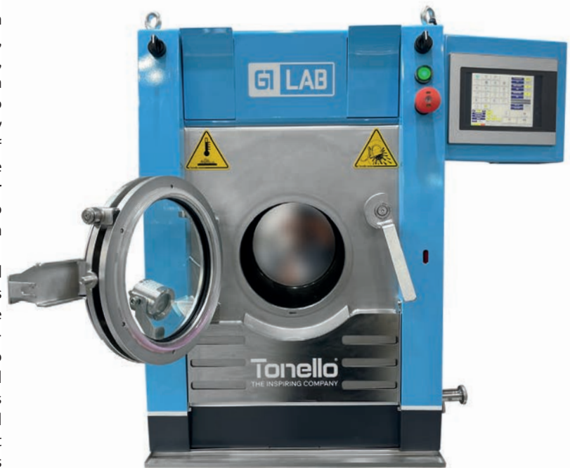
Italian denim processing machine maker Tonello displayed a lab-scale ultrasound garment-dyeing machine on its booth.
