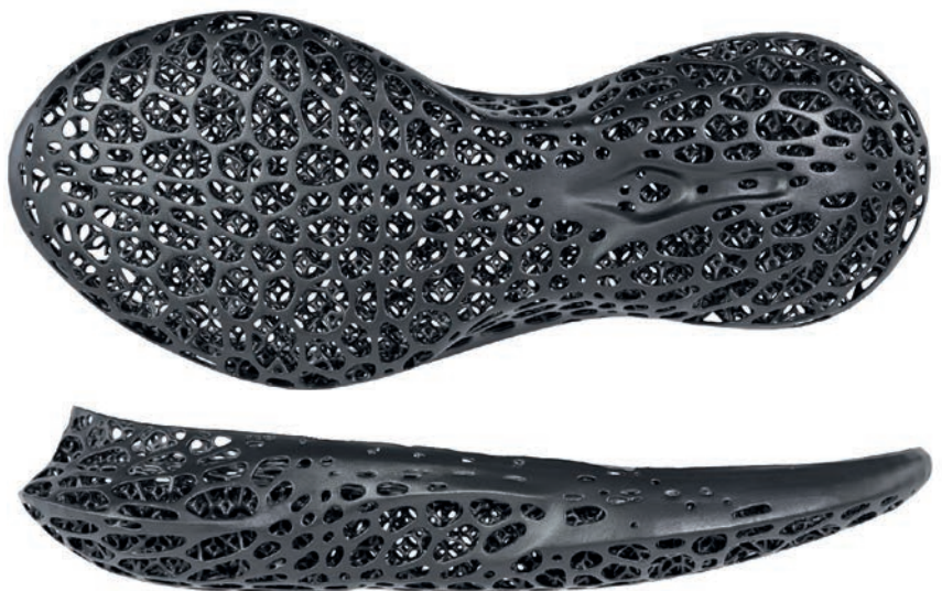
Made solely from BASF’s Ultrasint TPU01, the HP-printed parts consequently have an 80% reusability rate.
