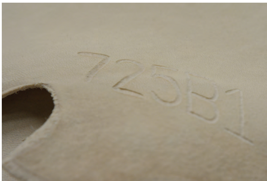
Spoor's system uses laser technology to mark hides with a unique alphanumeric code.
