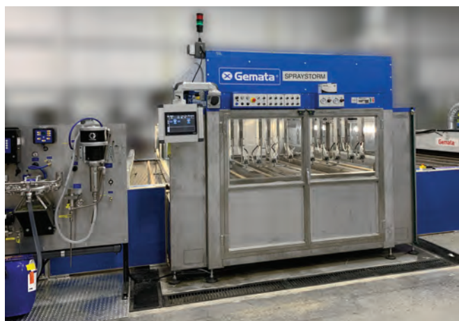
Housed in the space saving booth, linear carriage units are controlled by "Brushless" motors. Each arm can hold two guns, each with independent height and speed adjustment. ALL CREDITS: GEMATA
