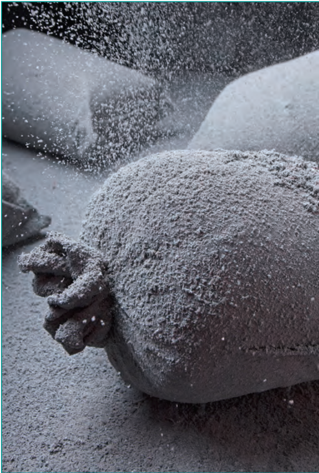
Leather waste is ground up to produce Cooloo's special spray coating.
