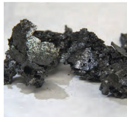
Biochar from LIFEGOAST leather shavings showed promising characteristics for use as a soil improver, replacement for cementitious aggregates, anode for lithium batteries and production of activated charcoal.
