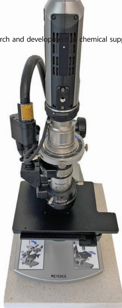
Among other equipment is a 4K Microscope, one of the first of a new deep resolution generation, allowing detailed analysis of defects, but also providing a complete investigative tool, enabling problem solving and control of the finishing, layer by layer.
