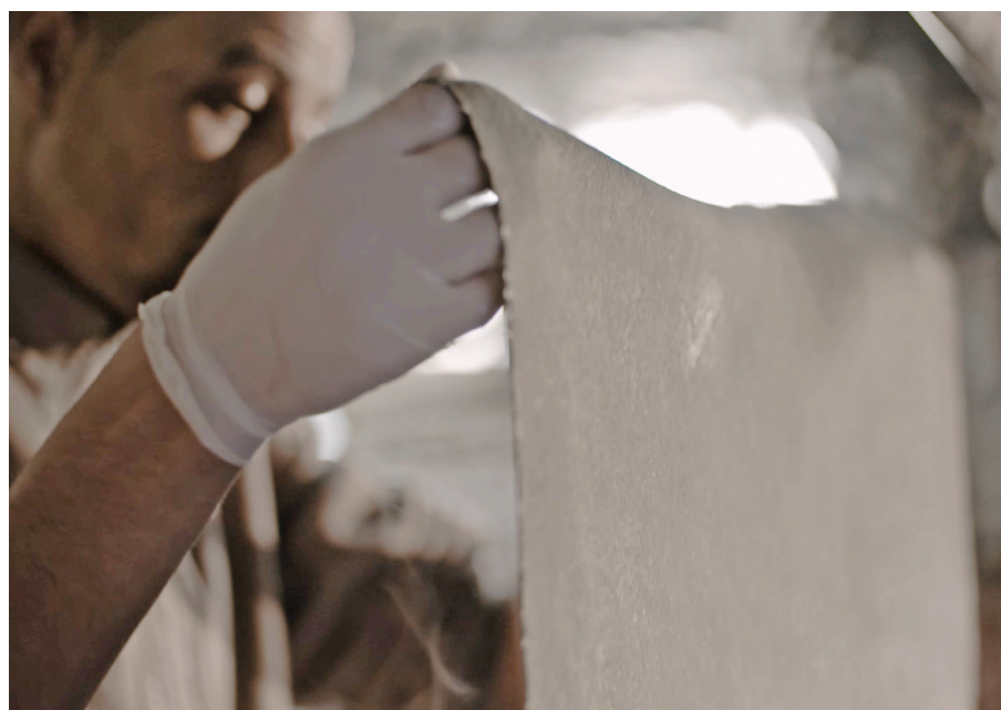
MycoWorks's Fine Mycelium process "engineers" mycelium as it grows, meaning that sheets are made to order for weight, shape and thickness. Credit: Laura Gutierrez / MycoWorks
