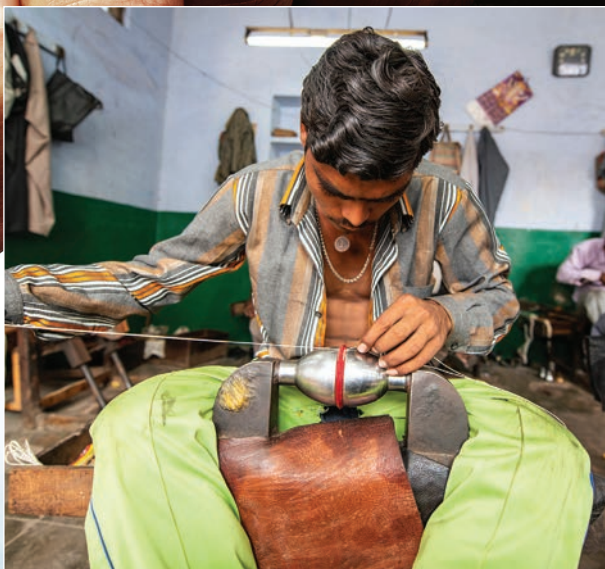
For the games played in England, the ball must be totally hand stitched. Firmly clamped together to create a raised seam, the ball is meticulously hand stitched to give the classic seam.
