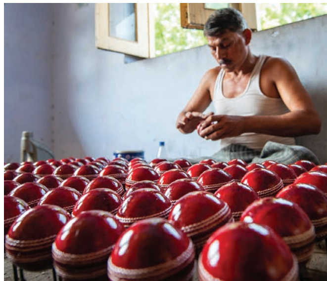
Cricket balls in the final stages of production, having a hand applied coat of polish.
