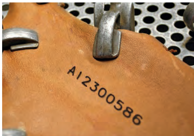
A clearer, more legible and less damaging mark from a laser system.
