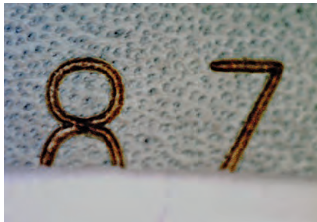
On the surface, where the fibres are more compact and vertical, Feltre's Leather Tattoo leaves a mark of between 0.05 and 0.1 millimetres in depth.
