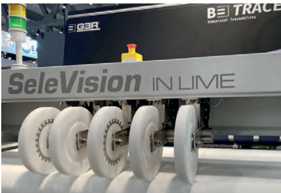
The BE Process system measures the effect on each individual hide of the processes it goes through in the tannery.
