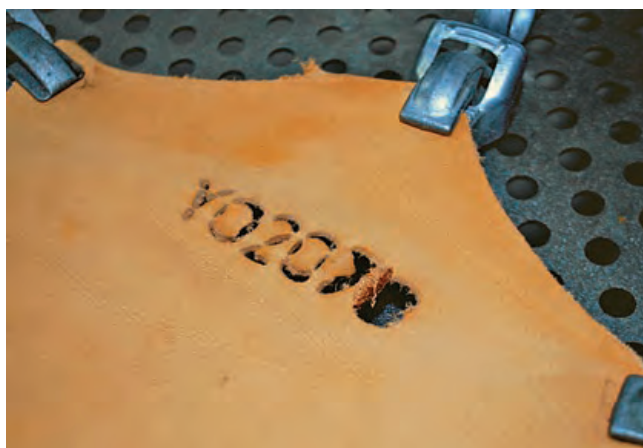
Damage caused by a marking system that perforates the hide.
