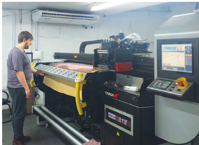
Around 20% of Courovale's finished leather goes through digital printing technology at the moment. It takes around 35 minutes to print a pattern on each side.
