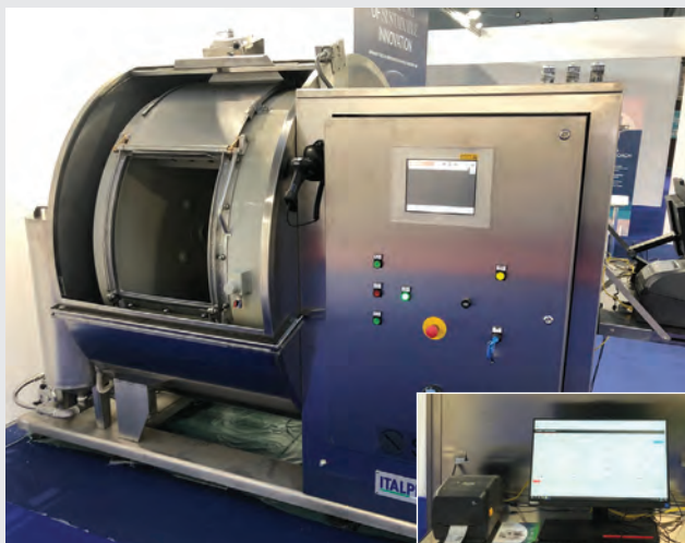
The drums program panel (right) is key in the monitoring of process performance and assessment of environmental impacts and costs.
