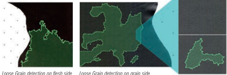
Loose Grain detection on flesh side (different hair density).
