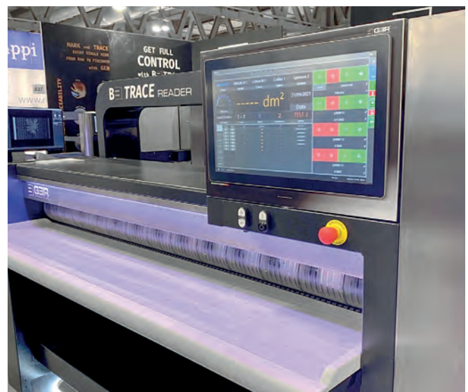
Conforming to the Measuring Instrument Directive (MID) 2014/32/UE, water resistant to IP65 regulations and working on the latest Microsoft Windows operating system, the EVA machine is far from window dressing. CREDIT: WTP
