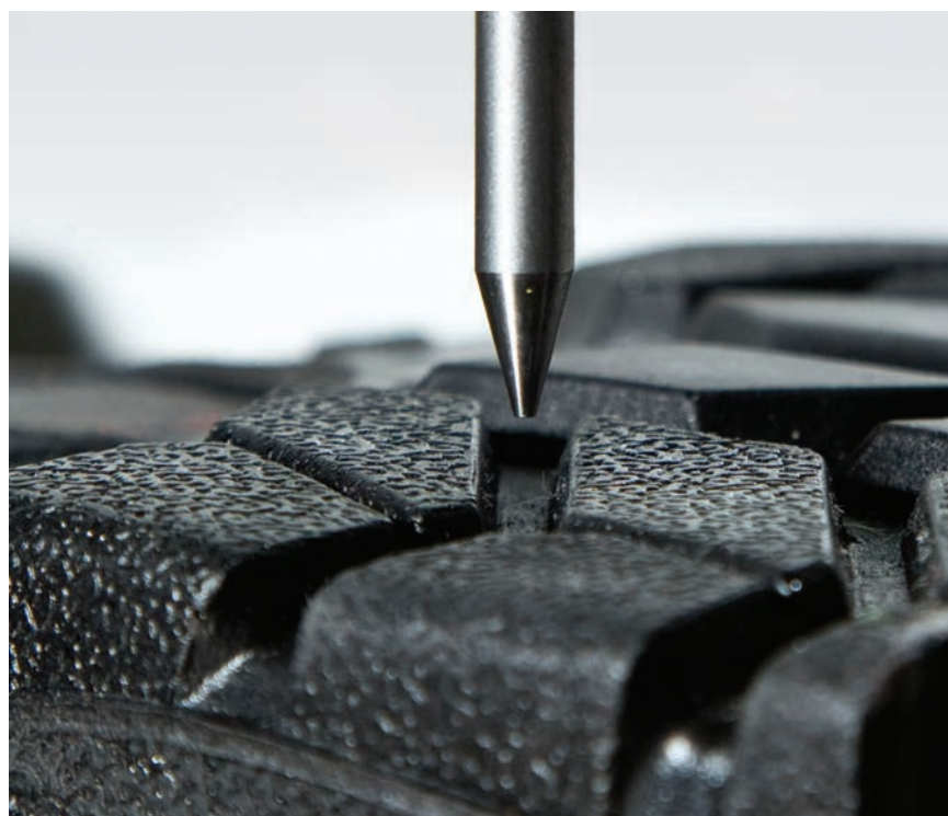
Nail penetration test on safety footwear.
