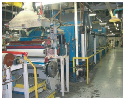
Materials are formulated and adhesive coated at Lowell, Mass. ensuring the same quality and performance wherever the tapes are cut. CREDIT IDEAL TAPE CO
