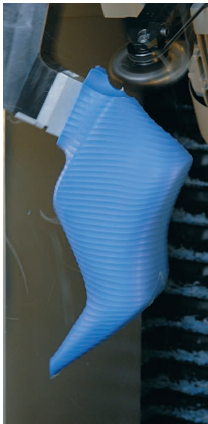
The Newlast NLS 1 milling machine holds the moulded blank at the top instead of at the toe and seat, then roughs and fine turns it in one sequence to produce a highly accurate finished last. CREDIT: NEWLAST GROUP
