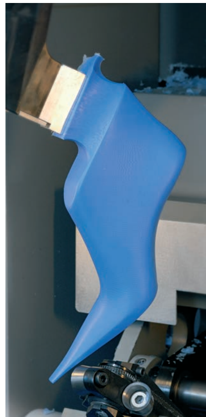
The Newlast NLS 1 milling machine holds the moulded blank at the top instead of at the toe and seat, then roughs and fine turns it in one sequence to produce a highly accurate finished last. CREDIT: NEWLAST GROUP
