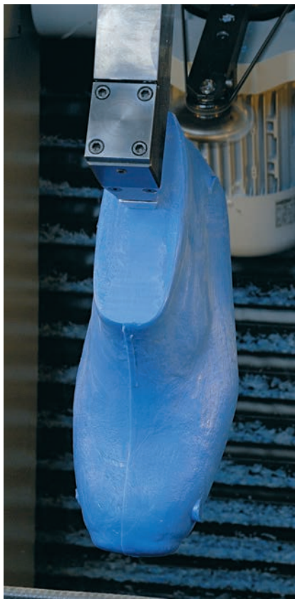
The Newlast NLS 1 milling machine holds the moulded blank at the top instead of at the toe and seat, then roughs and fine turns it in one sequence to produce a highly accurate finished last. CREDIT: NEWLAST GROUP
