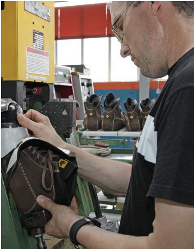
A technician applies a toe-cap to the upper of a workwear boot in the AMF factory in Guimarães, Portugal.
