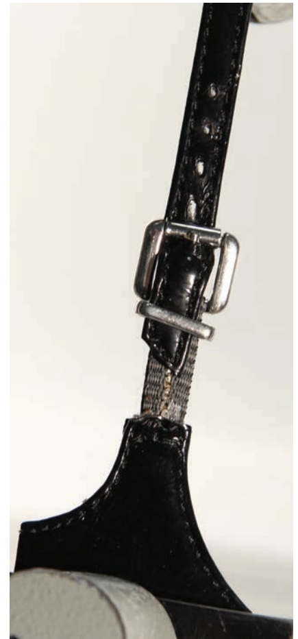
It is always preferable to test the strength of the complete buckle and strap assembly.
