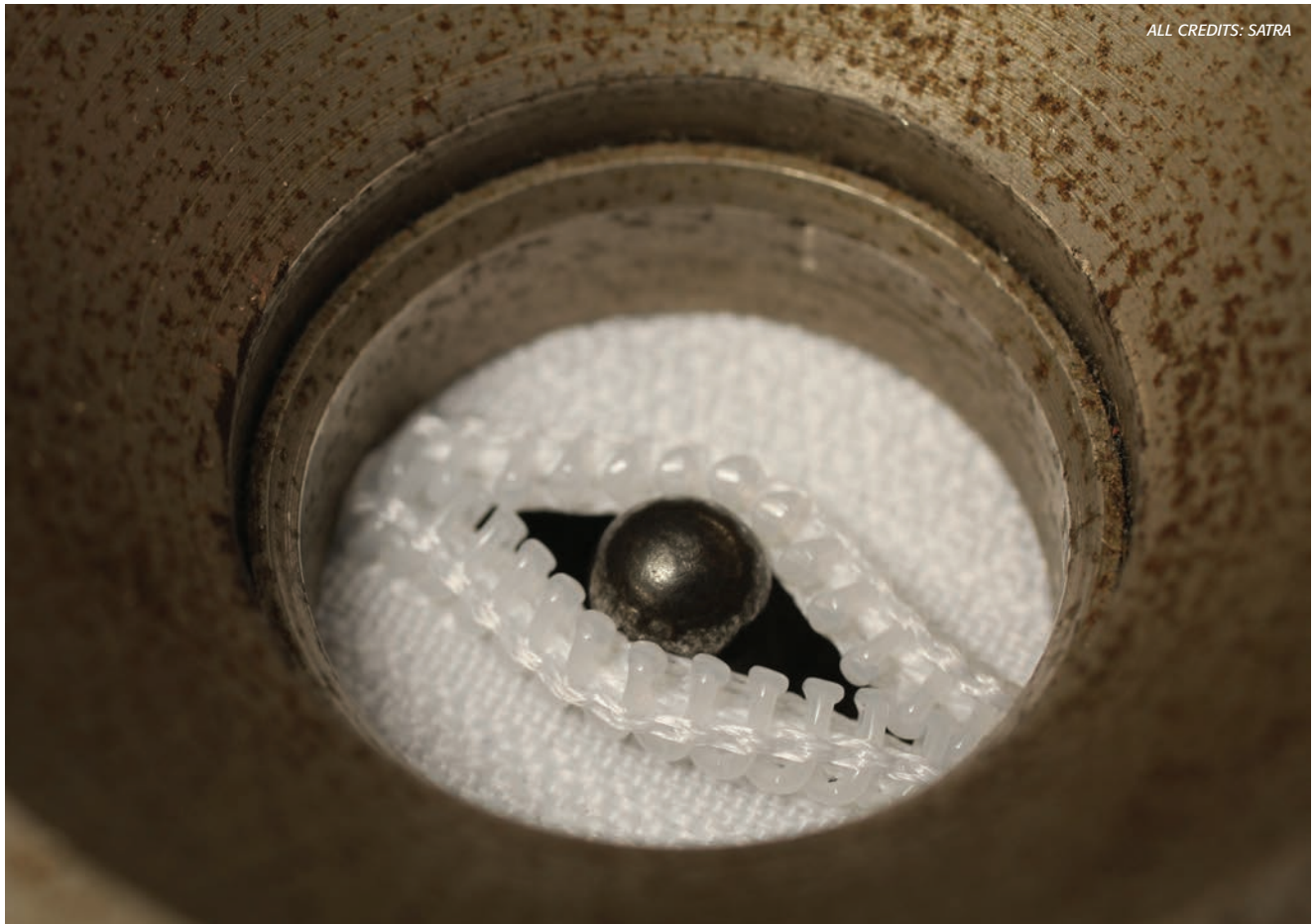
Resistance to bursting is a critical factor with zippers.
