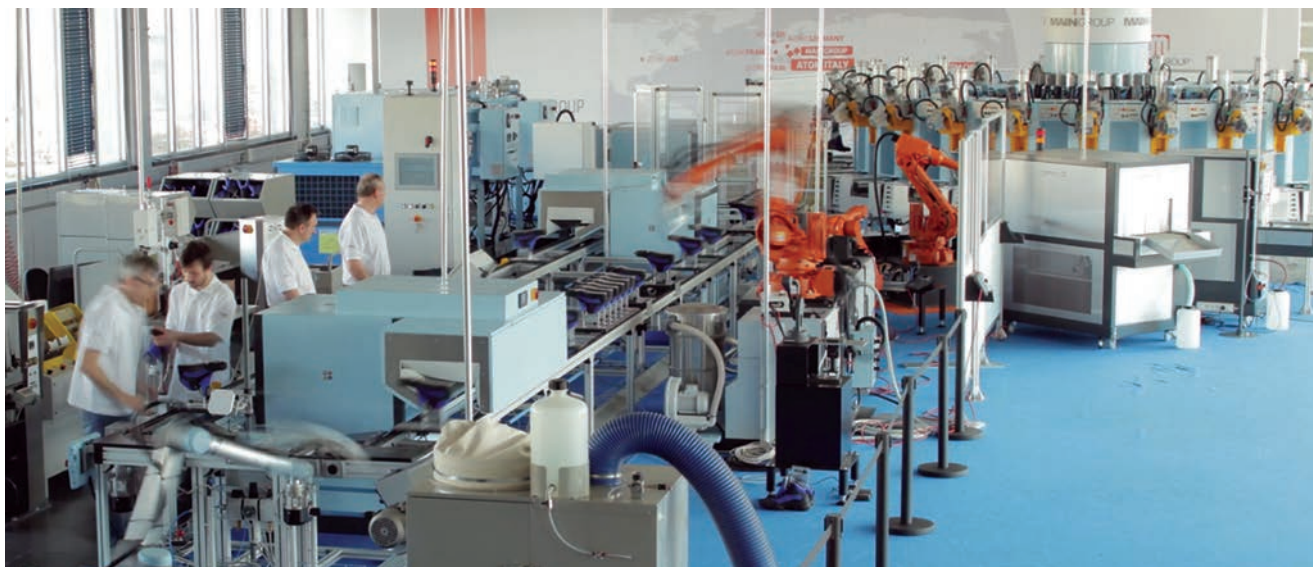
APP line for direct injection safety footwear typifies the new manufacturing concepts being worked on by ATOMLab.
