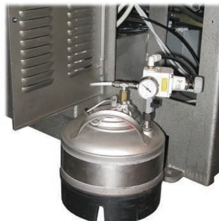
Special injectors are used for water-based adhesive on the Cerim K78TP. CREDIT: MOLINA E BIANCHI SPA
