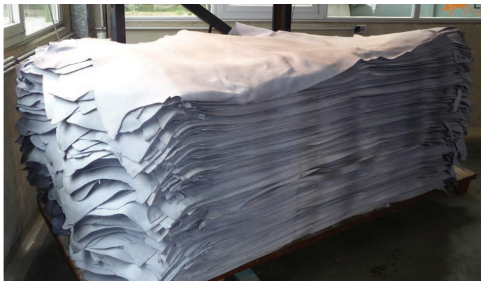
Most leather is now tanned to the wet blue state and sold on to be finished to specific needs. CREDIT: WTP
