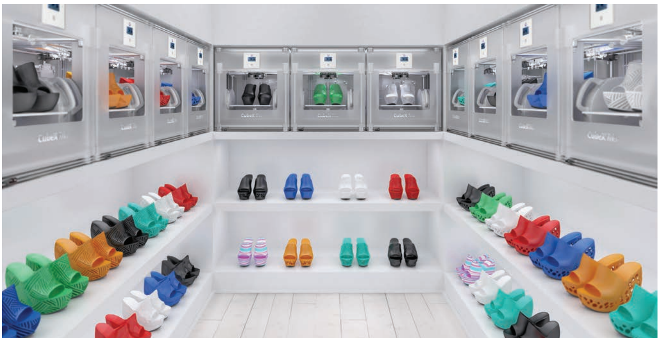
Fashion clogs produced on a 3D Systems machine showing the design and colour potential that is possible with additive manufacturing systems. CREDIT: 3D SYSTEMS
