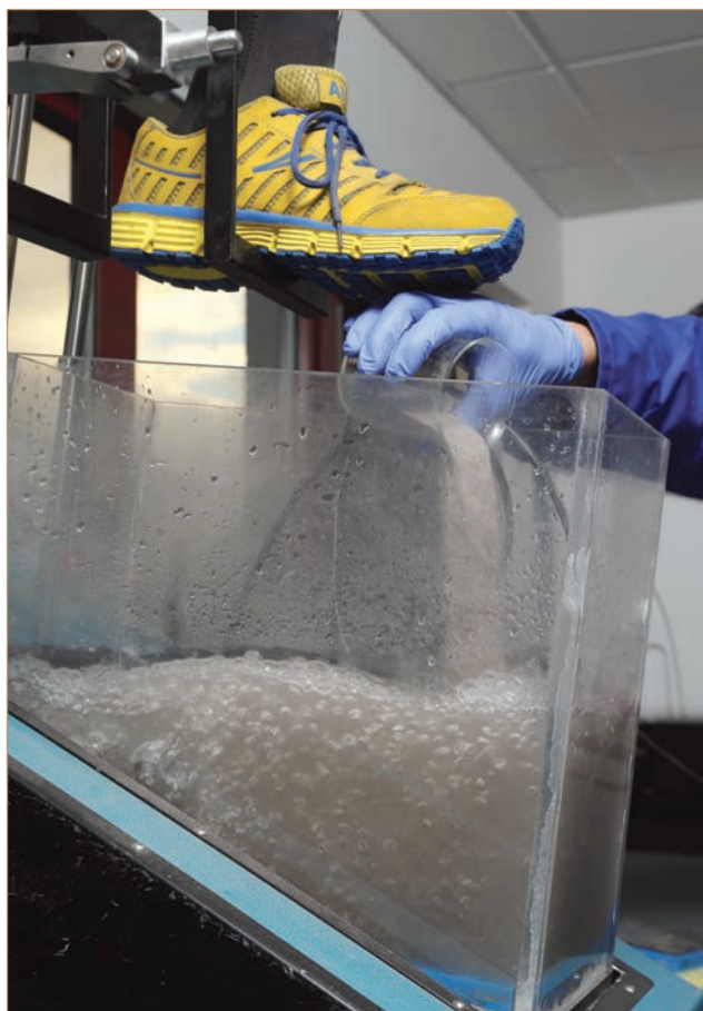
Aluminium oxide grit is kept in circulation by compressed air diffused through baffles in the bottom of the tank.
