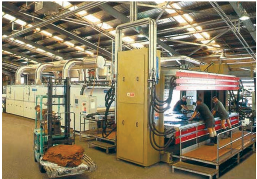
The machines in the tannery today can match those to be found in advanced technology companies. This vacuum drying machine at a tannery in Australia is used to extend and flatten skins before completion of the drying process. CREDIT: WTP
