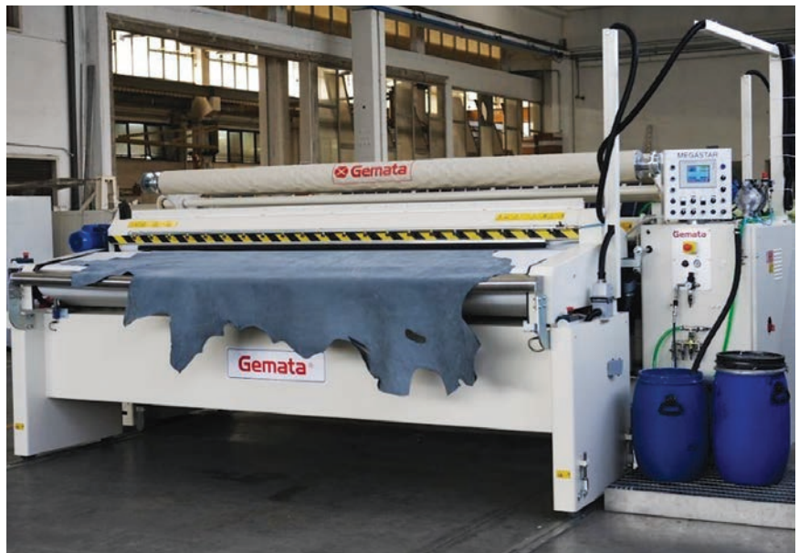
Sophisticated machines, such as this roller coater, provide tanners with multiple options to suit their production, similar to deciding what features you would like when buying a car. The options that can be added to the basic machine appear to be almost as numerous. CREDIT: GEMATA SPA
