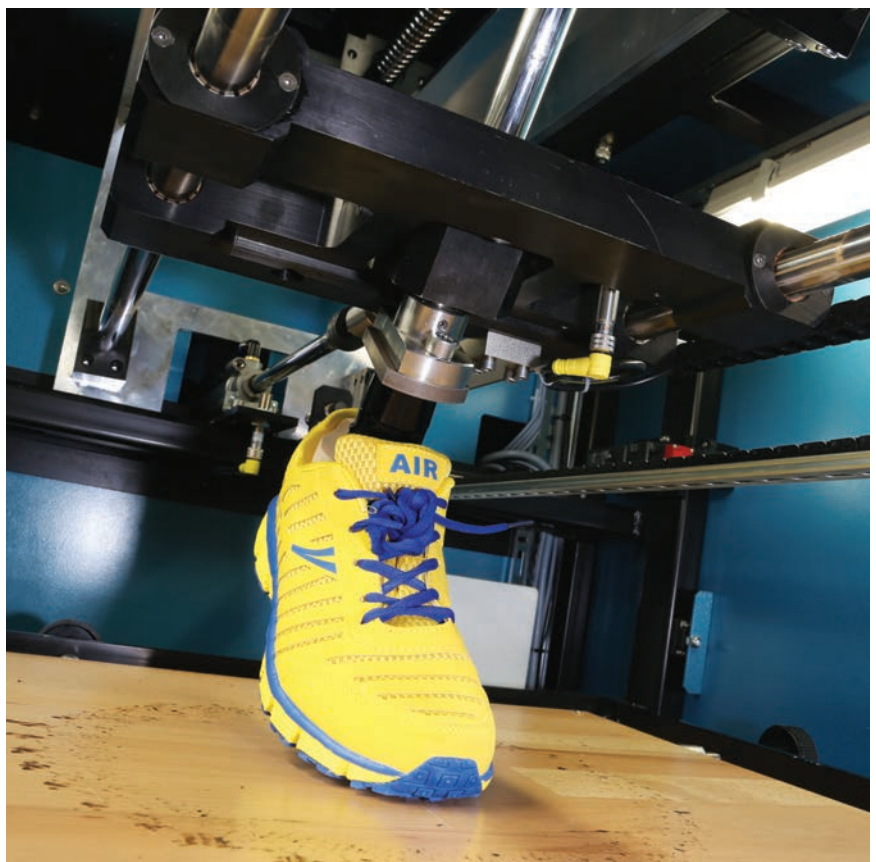
The STM 528 Pedatron accurately simulates real life wear patterns in a shoe.
