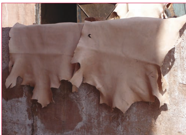
Mostly the leathers are tanned as "natural" due to its versatility. After tanning they are washed then slowly hang-dried tension free.
