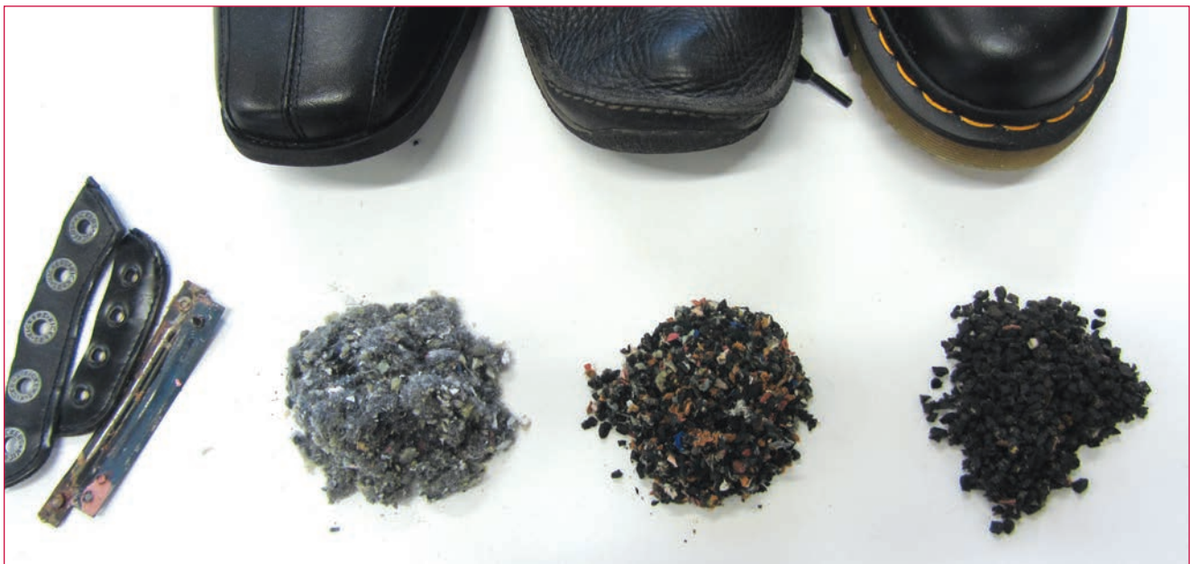
Leather-based shoes with high density rubber soles separated (left to right) into foam, textile and rubber again at 3-4mm average particle size.
