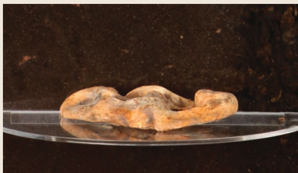
Figure 3. After 14 days degradation of the leather structure is profound. This compares to 31 days under natural composting conditions.
