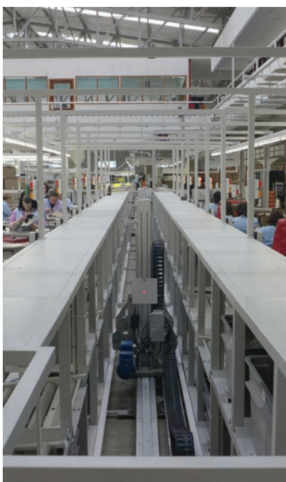
Robots shift materials to the stitching line.
