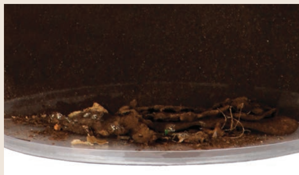
Figure 4. After 21 days the shoe has now totally disintegrated. This compares with 2 months under natural composting conditions.
