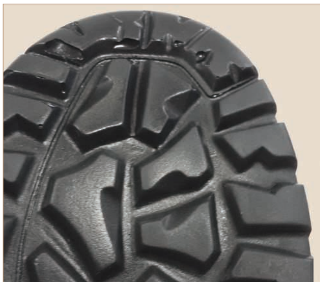
A PU sole made with a traditional injection system shows evidence of bubbles, flaws and has a less than perfect definition.
