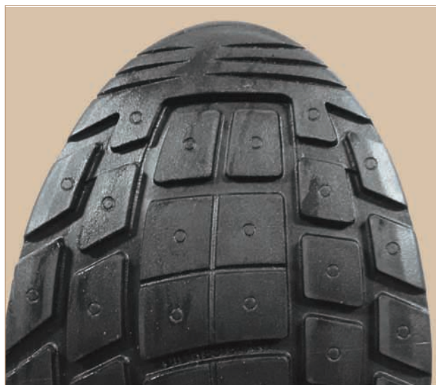
A PU sole made using the new improved system shows a distinct improvement in terms of both definition and overall surface quality.
