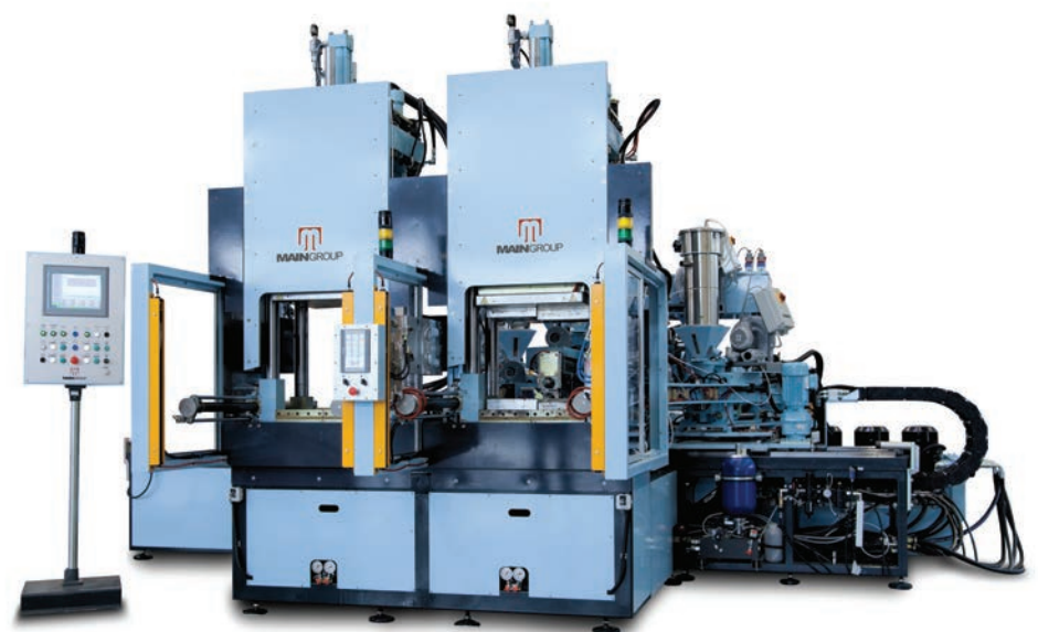
Main Group's E266 Evaluation EVA moulder is an example of the RCM concept.
