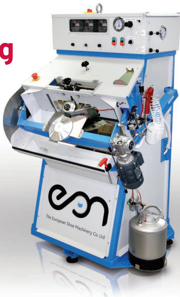
The EUHT heel and sole edge trimmer replaces two machines with one.
