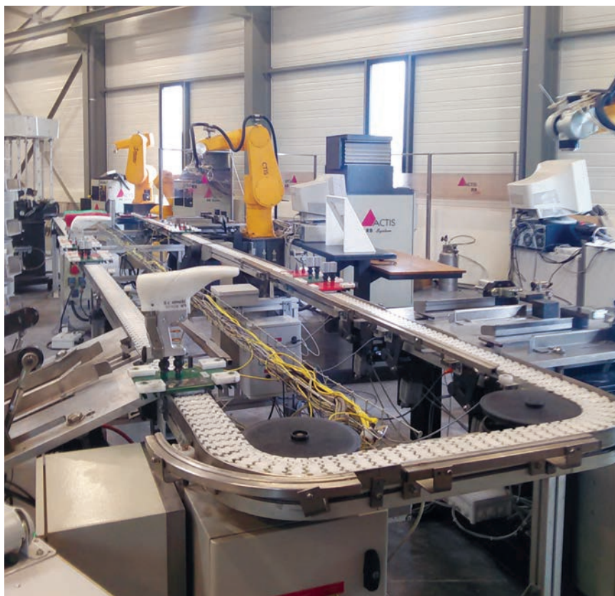
One idea, using automation to roboticise specific cells, has been to process soles and uppers on the same line.
