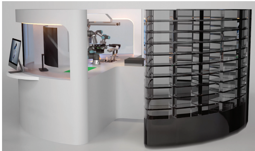
Concept design of a digital model of an ultra-compact shoe making machine that could be installed directly in a retail shop.
