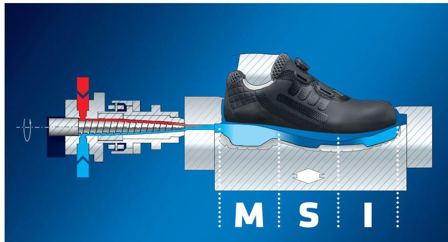
Multi Section Injection allows a high degree of customisation of midsoles in terms of hardness, softness and shock absorption.
