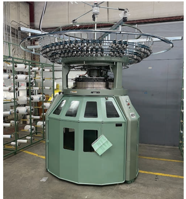
Faytex uses circular knitting techniques to create product from rPET and Repreve rPET yarns.
