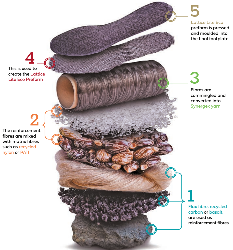
Figure 1: The five stages in creating a Lattice Lite Eco torsion plate.
