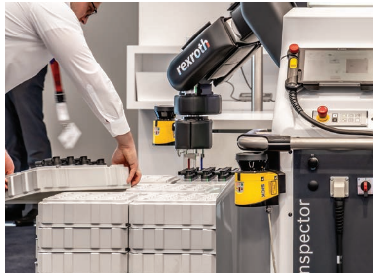
Cobots allow the close proximity of human operators.
