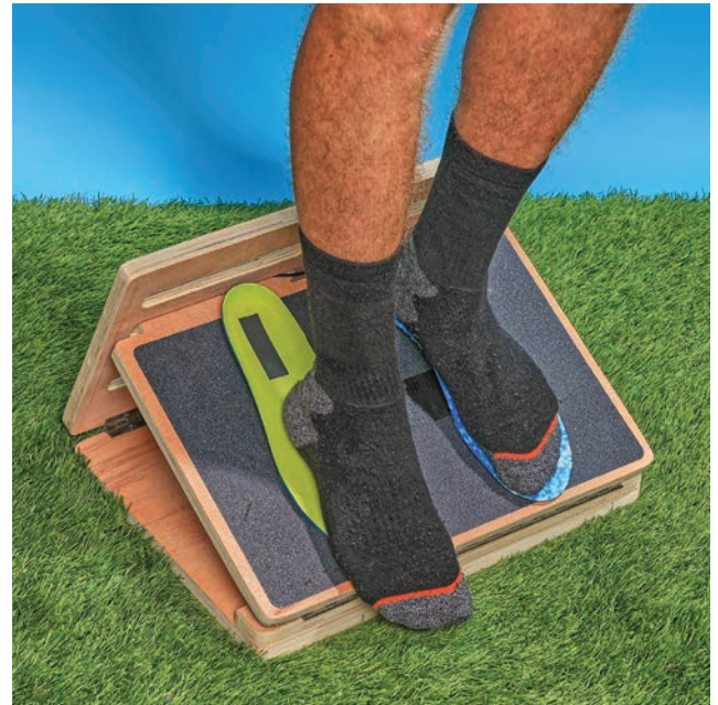
The Konnect insole on the right shows superior grip compared to that of the conventional insole on the left.
