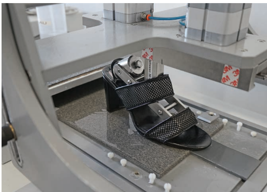
Testing a complete shoe for resistance to slipping.
