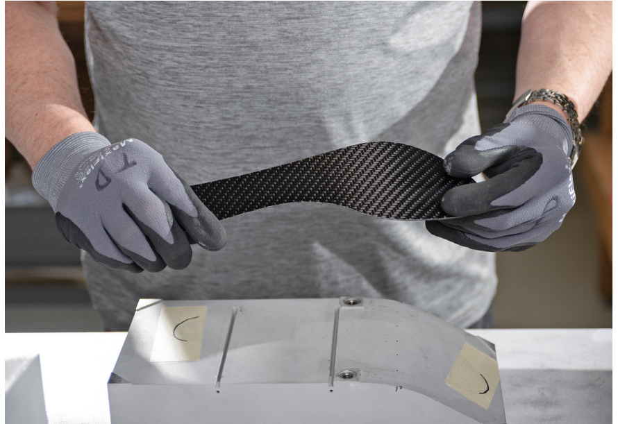
The material is stiff in one direction to provide underfoot protection, but high flexibility in the opposite direction.
