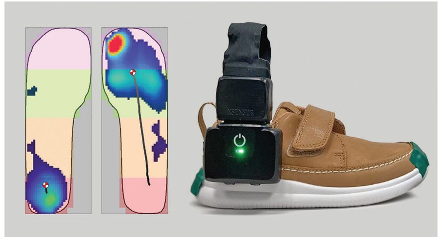
Clarks shoe with XSensor insole and screen shot of XSensor pressure software.
