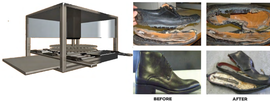
Figure 2 : Automatic disassembly of shoes using specially design cutting operation
