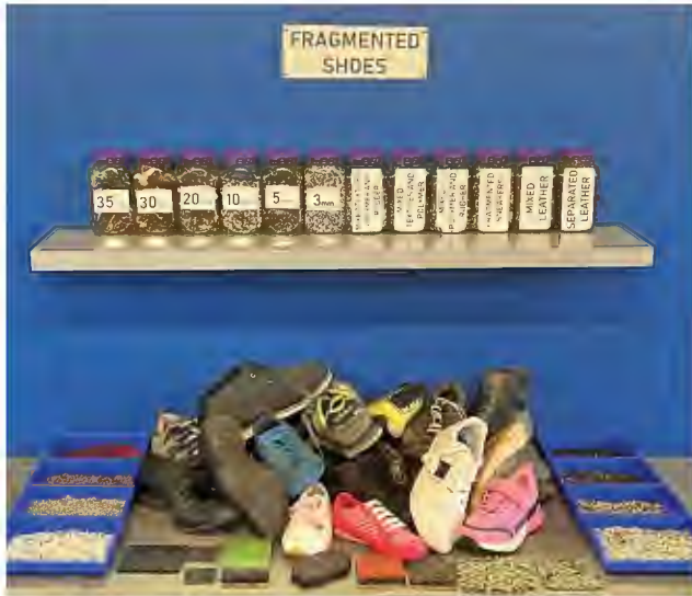
Figure 4 : Fragmentation and separation of footwear materials.
