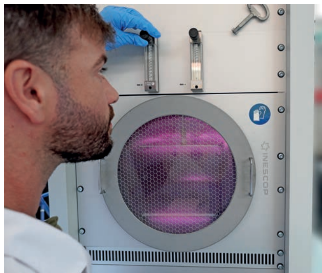
Silane monomer plasma beam in low pressure plasma equipment.
