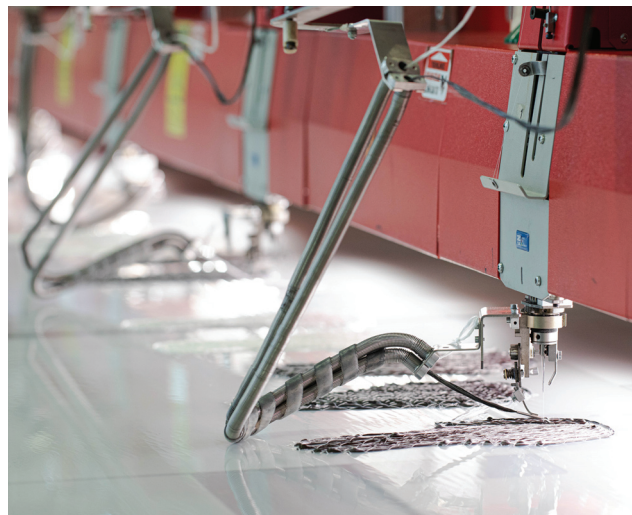
Lattice Lite Eco is a revolutionary fibre-laying technology that uses eco-friendly raw materials to create preforms without cutting or chopping fibres.
