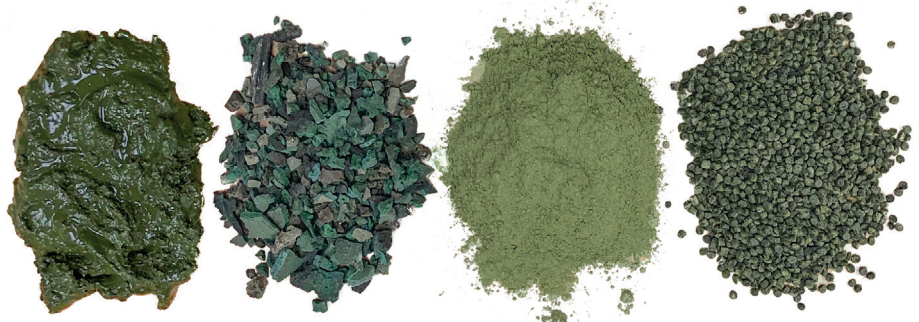
After harvesting, the initial sludge is dried into flakes, converted into powder form and combined with polymers and pelletised for use in a wide range of products.
