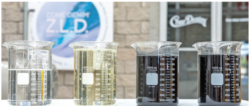
The factory’s effluent goes from a dark to a lighter shade of blue, then becomes yellowish before reverting back into clean water. PHOTO: CONE DENIM
