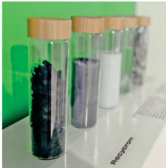
Officina39 grinds waste sorted by colour into a powder that is similar to a pigment.
